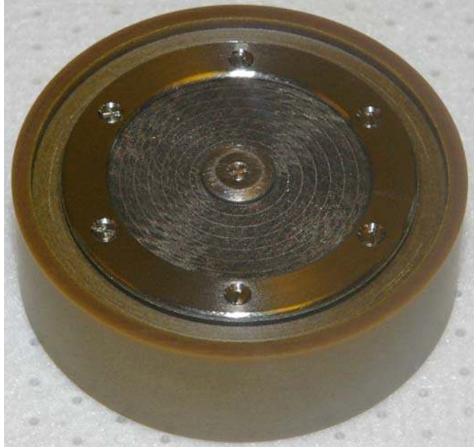
Figure 12.—Assembled oscillating-flow rig regenerator (stack of 42 disks).
