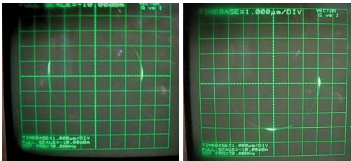
Fig. 37. One hundred mW power full transmitter measured constellations in BPSK and residual-carrier BPSK modes.
