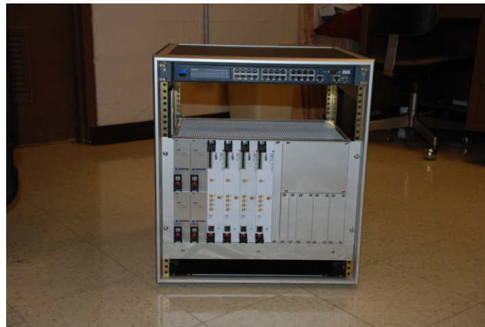
Figure 2.—Microwave sensor electronics, 24 GHz system, x4 channels.
