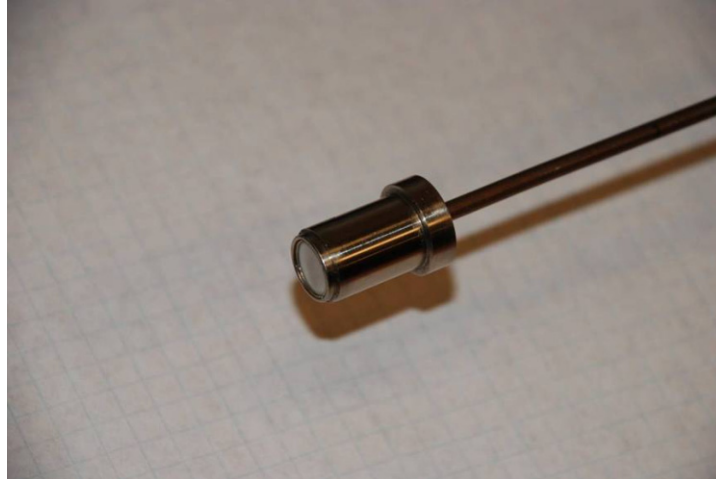
Figure 1.—Microwave blade tip clearance probe, 5.8 GHz.
