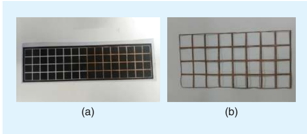
FIGURE 10. (a) A black-and-white plastic film mask, e.g., a negative image, was used to print the mesh-grid design on the copper sheet metal. (b) The final resulting 8 × 4-cell section of cloak. <AU: From where were these images obtained, and do you have permission from the source to use them?>
