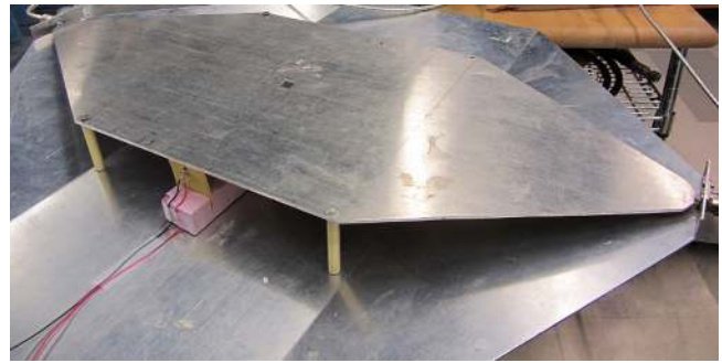
FIG. 3. Placement of SRR within open waveguide.
