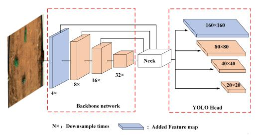
Figure 7. The model of feature extraction.
