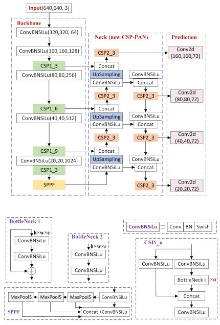
Figure 8. The configuration of the modified network.
