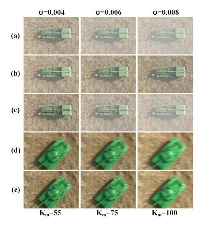
**Figure 14.** Pre-processed blurred images. (**a**,**d**) are the fog-blurred and motion-blurred images, (**b**,**c**) are the pre-processed images by the homomorphic filter [21] and FFA-Net [22] respectively, and (**e**) are the de-blurred images by DeblurGAN [23].
