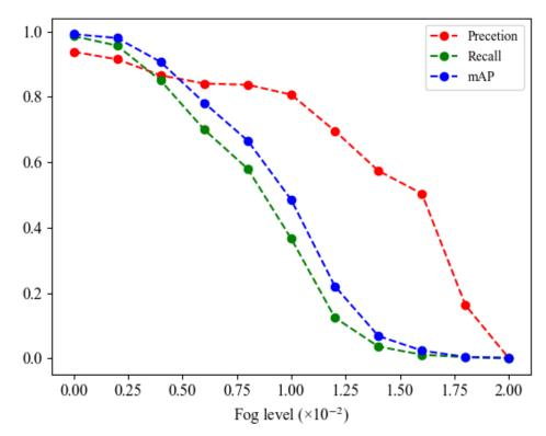
Figure 6. Detection accuracy of YOLOv5 on fog blur images.
