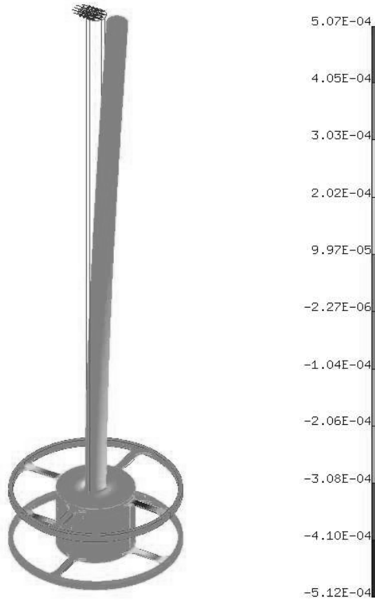
Fig. 3. FEA Force Sensor Strain Response to 1.0 N Radial Force
