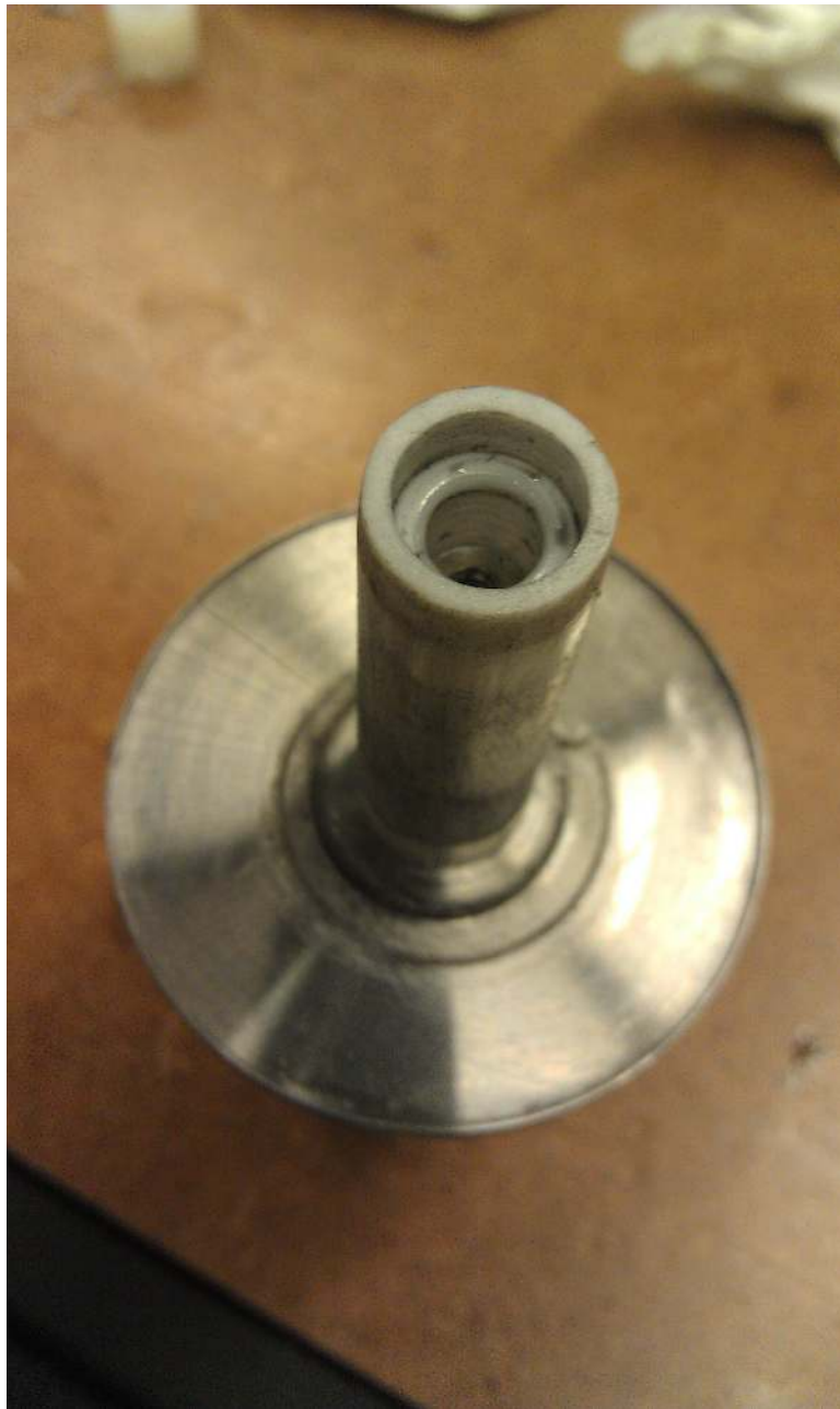
Figure A.15. Piston squeeze ring resting inside PTFE piston sleeve, Revision 02.
