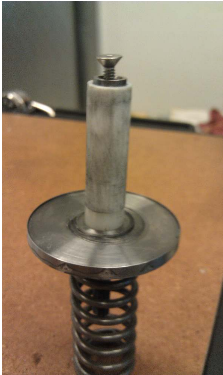
Figure A.17. Piston nut and screw installed, untightened, showing full piston assembly, Revision 02.
