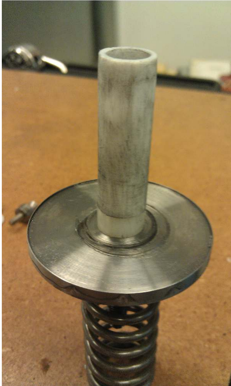
Figure A.16. Piston spacer on the bottom of assembled piston, Revision 02.
