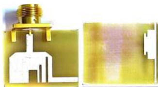
Fig. 3. Top and bottom of the fabricated proposed UWB antenna
