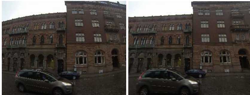
Fig. 1. An example of radially distorted image (Left) captured by a GoPro Hero3 camera and the undistorted image (right) using our method.
