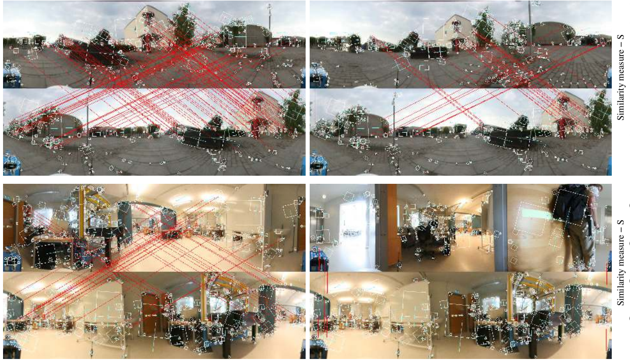
Figure 2: Examples of loop closure detection outdoors (top) and indoors (bottom). In the outdoor example the distance to the extracted features is larger than in the indoor example. Left: feature matches at the peak of the similarity value, S_{678,758} = 0.728 (top) and S_{7,360} = 0.322 (bottom). Middle: feature matches two steps (equivalent to \sim 3 meters distance) away, S_{680,758} = 0.286 (top) and S_{9,360} = 0.076 (bottom). The pose standard deviation \sigma_{x^{rv}} = \sigma_{y^{rv}} was estimated as 2.06\text{ m} (top) and 1.09\text{ m} (bottom), respectively, and the mean d_\mu as 0.199\text{ m} (top) and -0.534\text{ m} (bottom). Right: evolution of the similarity measure S against the distance travelled (obtained from odometry) together with the fitted Gaussian.
