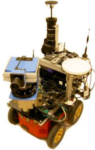
Figure 8: Outdoor robot used in this paper, equipped with a Canon EOS 350D camera and a panoramic lens from 0-360.com, which were used to collect the data, a DGPS unit to determine ground truth positions, and an LMS SICK scanner used for visualization and for obtaining ground truth.
