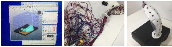
(a) 3D printing outer shell (b) Assembling: sensors, LEDs, Arduino (c) Final form with pressure dots at the back
