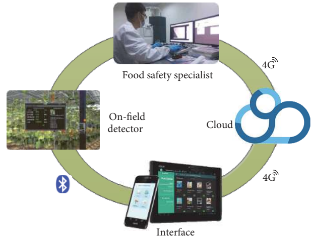
FIGURE 1: Overall view of the OP on-field detection platform based on IoT.
