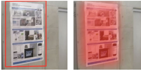
Figure 4: Highlighting of interaction points for context-based services. Instead of framing objects (left), we propose a soft border visualization (right) for less sensitivity to jitter and to reduce distraction of the user.
