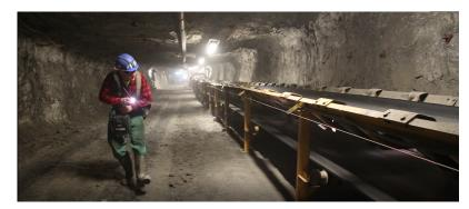
Figure 1. Conveyor belt route inspection in traditional form.
