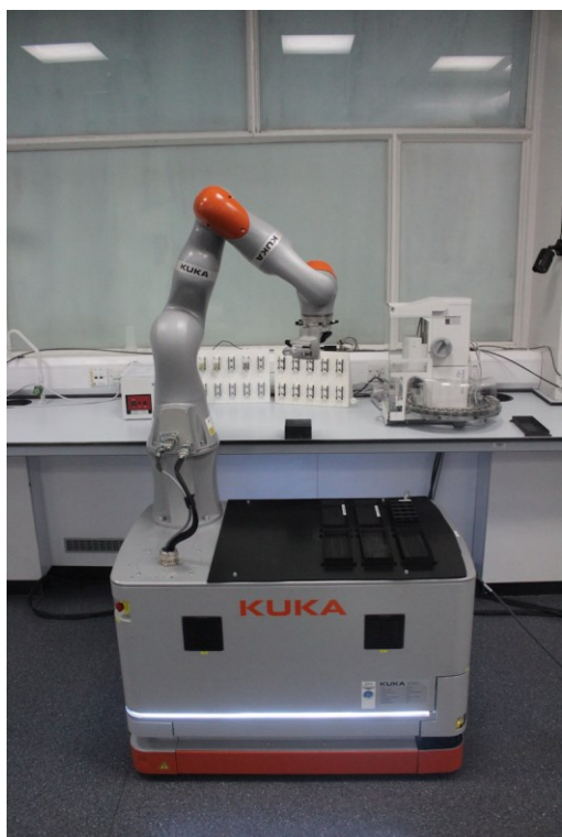
Extended Data Fig. 1. Mobile robotic chemist. The mobile robot used for this project, shown here performing a 6-point calibration with respect to the black cube that is attached to the bench, in this case associated with the solid cartridge station (see also Supplementary Fig. S11; Extended Data Fig. 3a).
