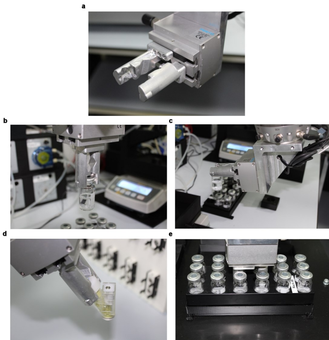
Extended Data Fig. 5. Multipurpose gripper used in the workflow. The gripper is shown grasping various objects. a , The empty gripper; b , gripper holding a capped sample vial (top grasp); c , gripper holding an uncapped sample vial (side grasp); d , gripper holding a solid-dispensing cartridge, and; e , gripper holding a full sample rack using an outwards grasp that locks into recesses in the rack. The same gripper was also used to activate the gas chromatograph using a physical button press (see Supplementary Movie S3; 1 min 52 sec).
