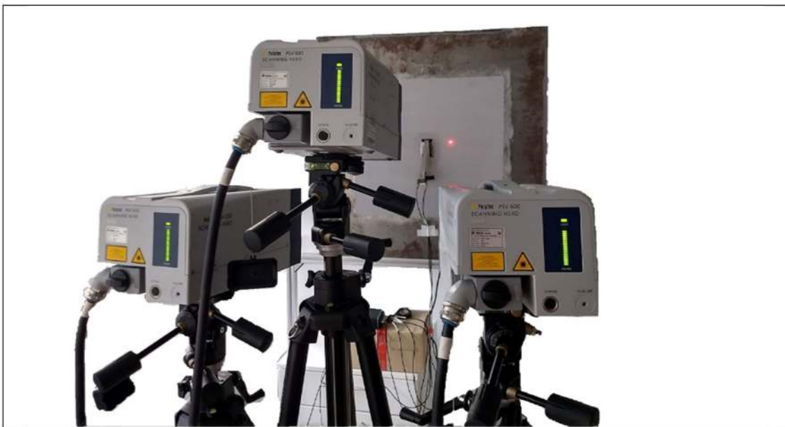
Fig. 9 Photograph of the setup for the wave propagation measurements by 3D laser Doppler vibrometry (Color figure online)
