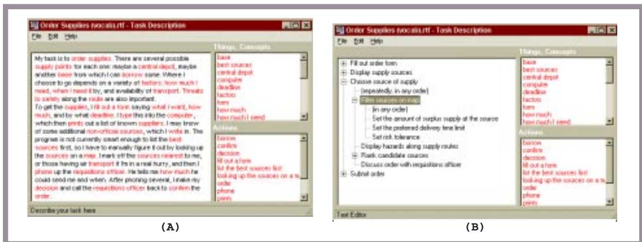
Figure 3. Mobi-D's user-task elicitation stage: (a) an informal task description, followed by a list of key items (boxes at right) and (b) a formal task outline, generated with help from the developer.
