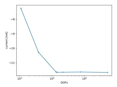
**Figure 8.** Convergence of the current with respect to the number of degrees of freedom (DOFs). Note that for a large number of DOFs, numerical issues may arise due to the small size of individual elements.
