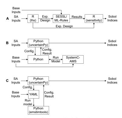
**Figure 4.** Schematic of the generated code for the three SA experiments for **(A)** the Wnt signaling model, **(B)** the battery model, and **(C)** the electric fields model. The experiments take the user-given base inputs and SA inputs and produce Sobol indices as outputs.
