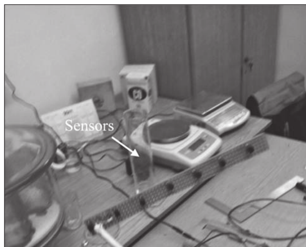
Figure 3 Sensors for pavement temperature measurement at a specified depth: sensors DS18S20 before being set in asphalt
