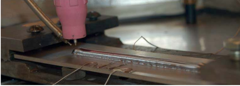
Figure 36. TIG-torch in argon chamber after depositing of the third layer.
