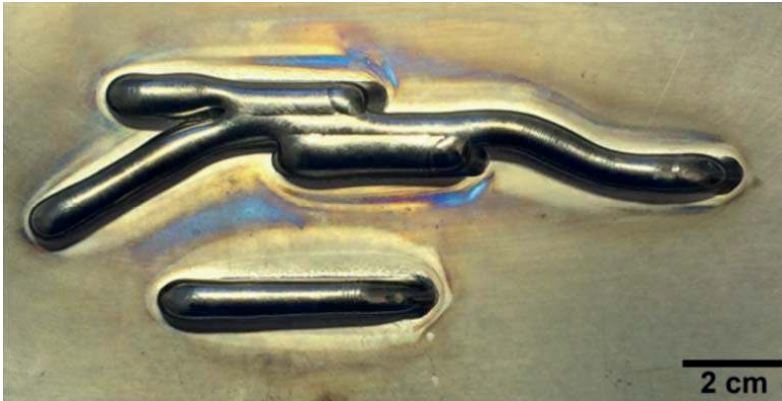
Figure 38. TIG wire feed deposited wall features in Paper D .
