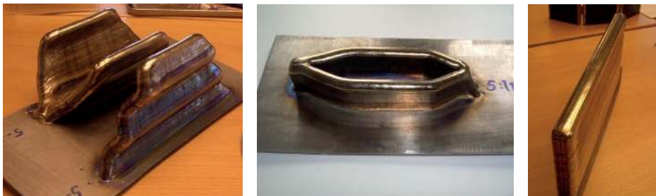
Figure 4: Different geometries built with GTAW metal wire deposition.
