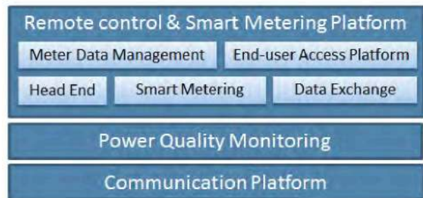
Fig. 6 Modules of the power quality monitoring and the remote control and smart metering platform
