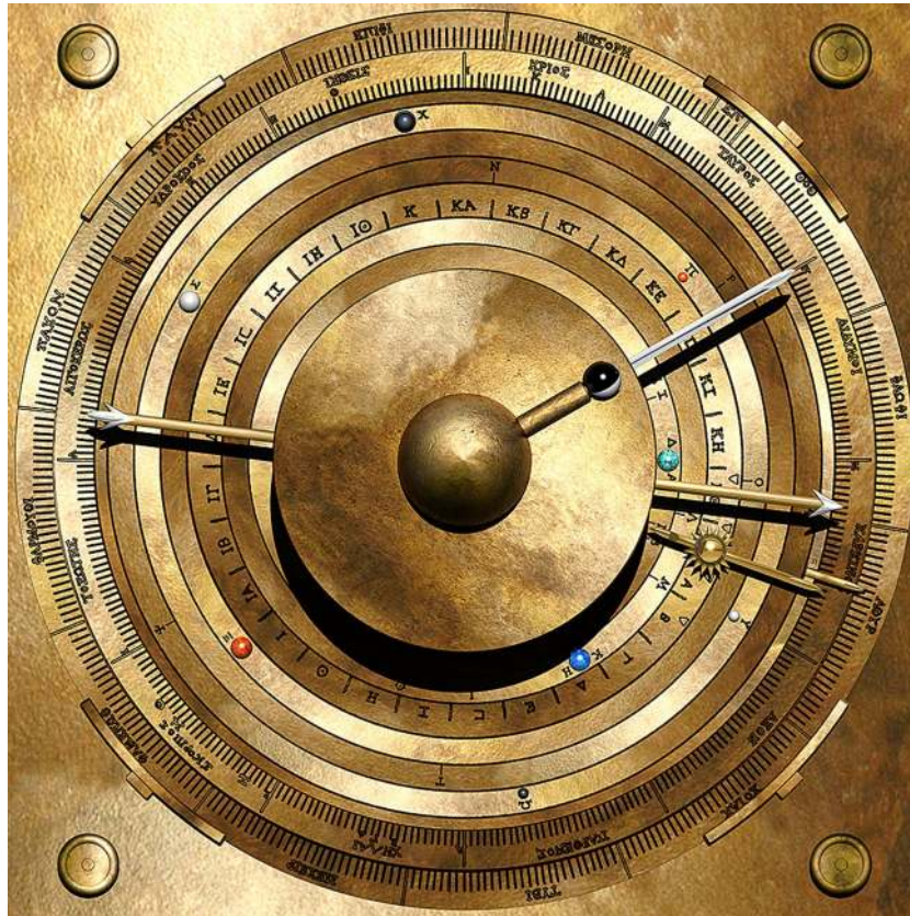
Figure 7. Computer model of the cosmos display. In the centre, the dome of the Earth, the phase of the Moon and its position in the Zodiac—then rings for Mercury , Venus , true Sun , Mars , Jupiter , Saturn and Date , with “little sphere” markers and smaller markers for oppositions. Scale marks and index letters for the synodic cycles of the planets are inscribed on the planet rings. Surrounding these, the Zodiac and the Egyptian Calendar 2 . The true Sun ring has a “little golden sphere” with “pointer”, as described in the BCI 9 . When the Moon and Sun pointers coincide, the Moon sphere shows black for New Moon; when the pointers are on opposite sides, the Moon sphere shows white for Full Moon 10 . The Head of the Dragon Hand shows the ascending lunar node ; the Tail of the Dragon Hand shows the descending node . Small triangles on the true Sun ring, near the pointer, show wider and narrower eclipse limits. Eclipses are possible if the Dragon Hand is within these limits. When the Moon pointer is before the Head of the Dragon , the Moon is South of the node; after, it is North of the node—conversely for the descending node . A Date pointer is attached to a narrow date ring, showing the date in the Egyptian calendar 2 .
