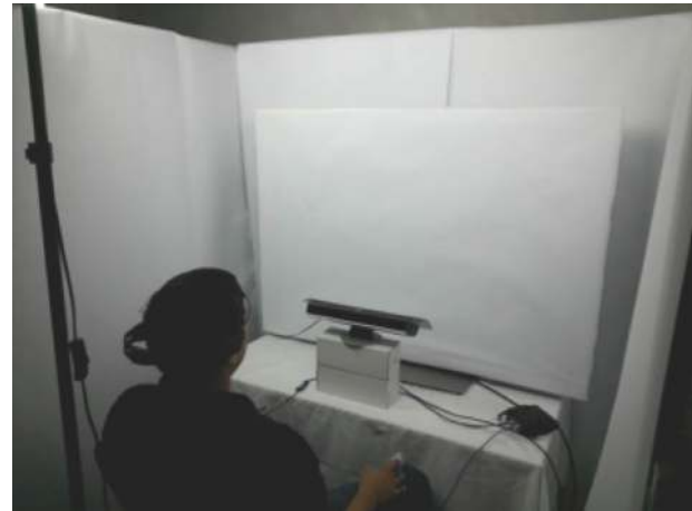
Figure 2: Experiment setup. The eye-tracker was placed between participant and wall/ TV; the computers to log all measurements were located out of the participant's sight next to the cubicle. Lamps as illumination sources were placed on tripods behind the participants about 40 cm above the participants' heads. This figure shows the configuration as it was used for part 1 of the experiment.
