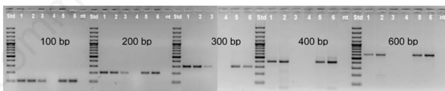
Figure 1. Control gene PCR for the assessment of amplifiability and integrity of DNA samples. Five control genes exons and the five primer sets for obtaining PCR products of 100, 200, 300, 400, and 600 bp 9 . 100bp ladder marker, samples from cancer patients 1-4; healthy controls 5, 6 and no template control, primer used as described in van Dongen et al. 2003.
