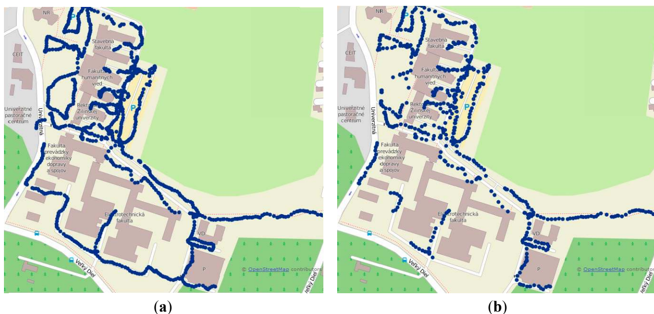
Figure 8. Outdoor radio maps for (a) GSM and (b) Wi-Fi displayed on Open Street Map.
