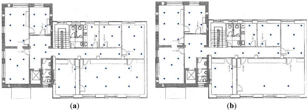
Figure 9. Indoor radio maps for (a) GSM and (b) Wi-Fi displayed on a plan of the building.
