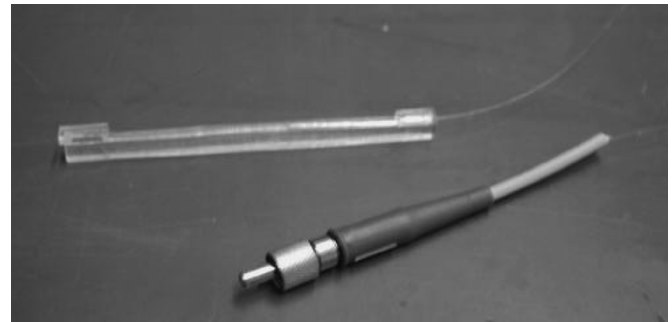
Fig. 6. PDMS waveguide interfaced to silica fiber.
