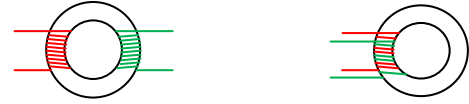
(a) Windings on both sides. (b) Windings on one side. Fig. 3. Two different coiling methods of the transformer.
