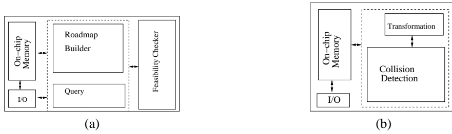
Fig. 3. Motion planning processor (MPP) in different configurations: (a) motion planning configuration, feasibility checker can be specified depending on the problem, e.g. collision detection or potential energy computation, (b) dedicated collision detection configuration.
