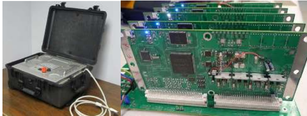
Fig. 5. The MRI robot controller (left) is a fully shielded enclosure containing the piezoelectric motor drivers, power supplies, and fiber optic communications in a portable case. The custom-developed piezoelectric motor controller driver boards (right), shown in the 5-axis configuration on a backplane that resides in the shielded enclosure.
