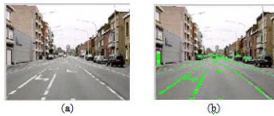
Figure 7. Lane Detection. (a) Original Image, (b) Lane Detection shown in green color
