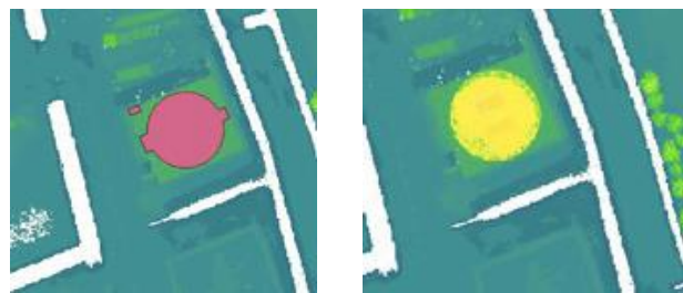
Figure 4. The BAG building on the left has no height, because the relevant point heights are classified in AHN as “ground points” (right)
