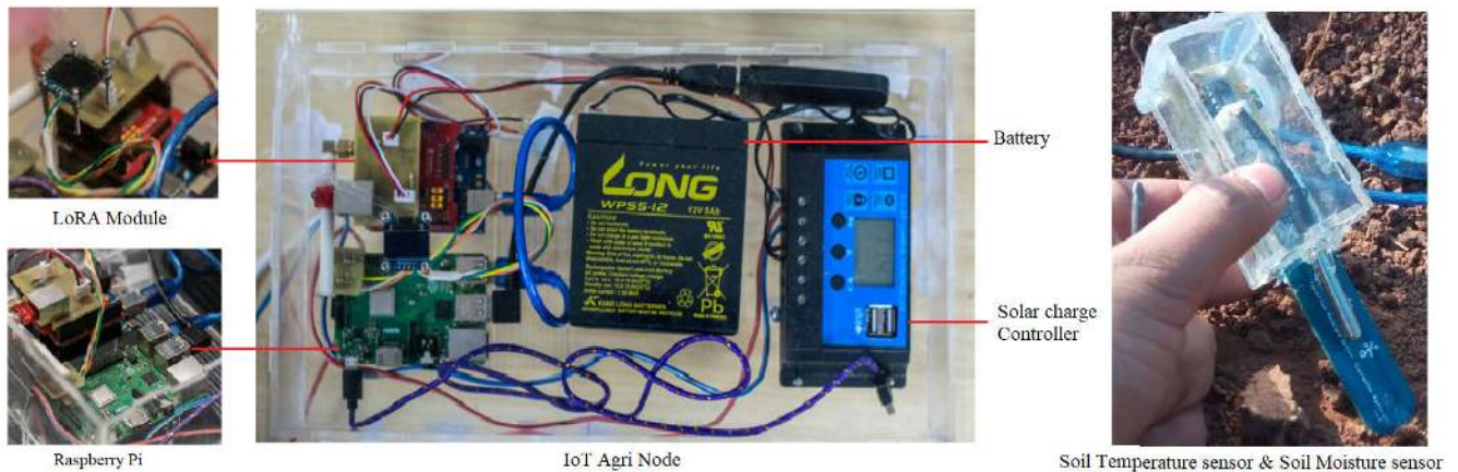
FIGURE 4. IoT Agri Node with its components.
