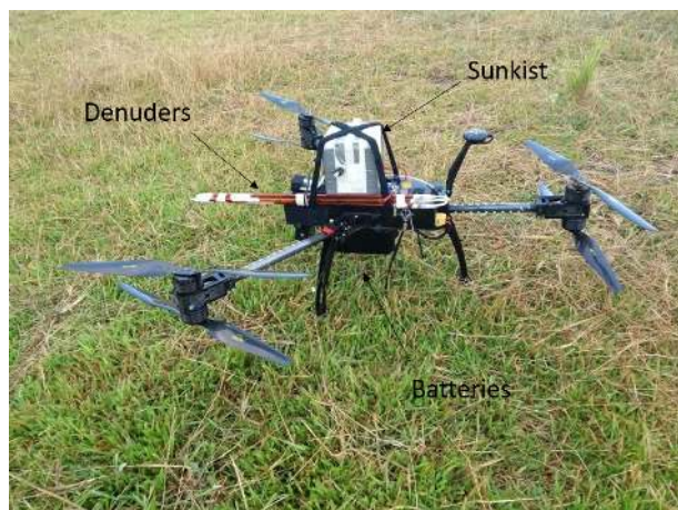
Figure 6. Drone-based denuder sampling setup and SO 2 sensor (Sunkist).
