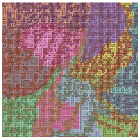
FIGURE 18. The spanning tree and coverage path of each robot in each sub-area.
