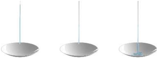
Fig. 12. Reduced-liquid flow and dripping on a single strand. Left: No reduced-liquid flow. Center: Reduced-liquid flow without dripping; the liquid flows towards the tip and disappears. Right: Reduced-liquid with dripping enabled.
