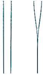
Fig. 6. Two wet hairs held close and then pulled apart. Left: Hair strands freely separate without cohesion. Right: Cohesion forces cause hair strands to adhere. Note: for better visibility of small-scale illustrative examples in paper images (only), the radius of hair and reduced-liquid have both been scaled up.
