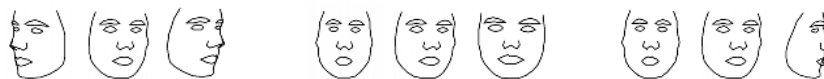
Figure 8: First three modes of shape variation for a view-context based nonlinear PDM. The range of variation is set to -1.5\sqrt{\lambda_i} \leq b_i \leq 1.5\sqrt{\lambda_i} .
