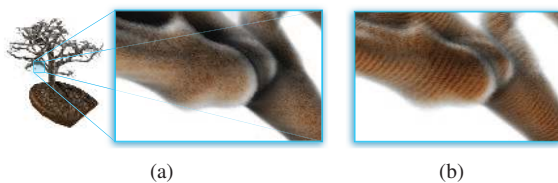
Figure 14: Visualizations of the bonsai dataset: slice-based volume rendering using a view-aligned slice stack (a) and using a half-angle-aligned slice stack (b).
