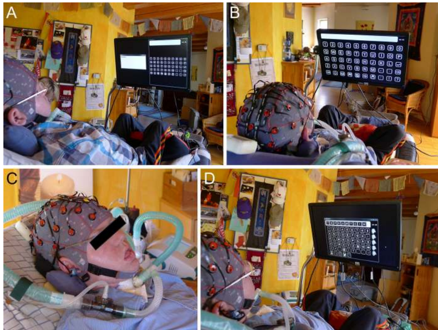
FIGURE 3 | End user 4 during testing of the prototype. In (A) the split screen mode is shown. In (B) the spelling matrix is displayed in full screen mode. The selected symbols were displayed in the line above the matrix such that the user received feedback although the corresponding application window for spelling was not inside his field of view. (C) depicts a close-up of the user and the electrode cap and in (D) the window size of the spelling matrix is adjusted to fit the application window size of his conventional software (dasher) used for communication. End user 4 gained only rudimentary control over the spelling application and did not test the other applications. Pictures are published with consent from the participant and his legal representative.
