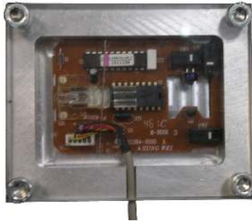
Fig. 3. Assembly product: a base plate, one electronic part, a wiring cable, a plastic cover and four screws
