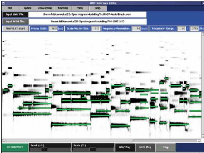
Fig. 9. Screenshot of the GUI editor we implemented to create the ground truth data set of note pitches, onsets, and durations. The note events of the supplement MIDI data included in the RWC database, which are not temporally aligned with the corresponding real performed signal data, are displayed as rectangular objects over the spectrogram of the real performed signal. We are then able to edit the rectangular objects to align carefully the onset and offset times according to the background spectrogram.
