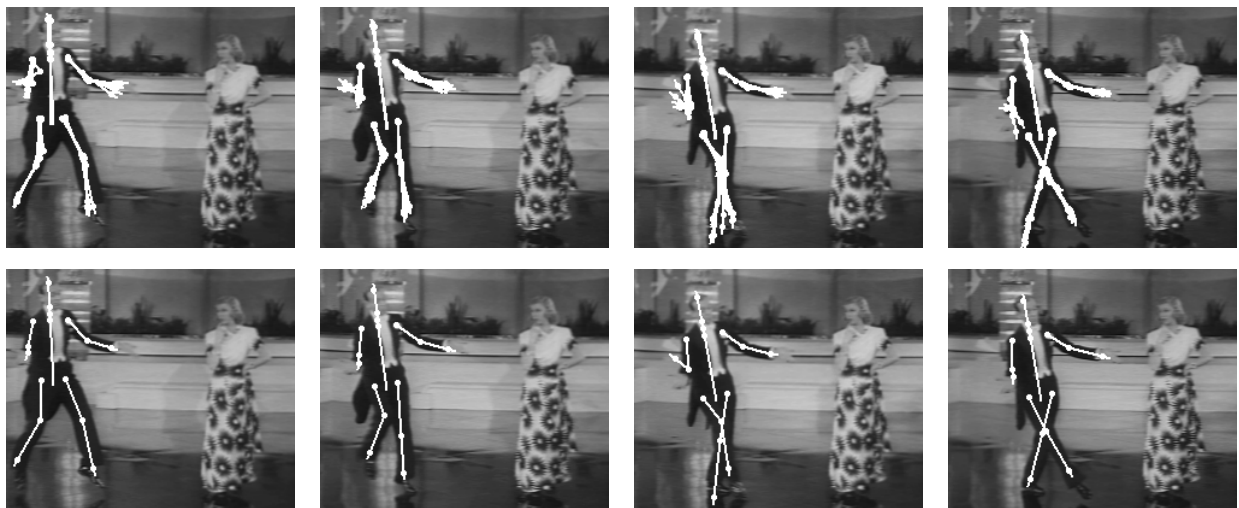
Figure 4: Mode-based Multiple Hypothesis Tracking Results. Top row: the multiple modes of the tracker are shown. Bottom row: the dominant mode is shown, which demonstrate the ability of the tracker to handle ambiguous situations and thus survive the occlusion event.
