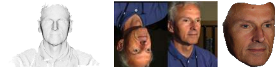
Figure 1: (left): Raw mesh output from the 3dMDface software. (middle): Texture image from two angles captured by the 3dMDface cameras. (right): The scan and texture densely registered to the 3D model.
