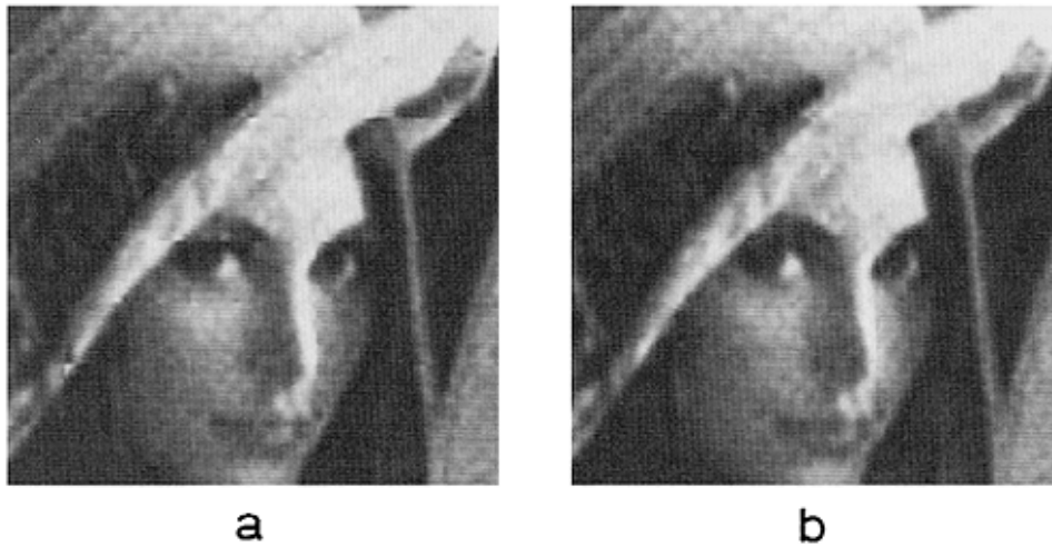
Fig. 9. The multiresolution spline used to remove block boundaries from a block transform encoded image. Figure 9a shows an image which has been block transform encoded at a rate of 0.5 bits per pixel. An 8 \times 8 array of blocks is shown, each containing a 16 \times 16 array of pixels. Blocks were treated as separate, nonoverlapped images to obtain the splined result shown in Figure 9b. Image quality remains low because of the very low bit rate of the code, but the perceptually prominent block boundaries are almost completely eliminated.
