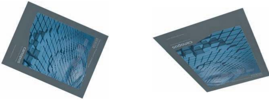
Fig 1. Two images of a planar object, taken from different viewing angles with a pinhole camera, are connected by a projective transformation, also called homography.
