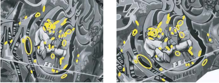
Fig 2. Affine covariant neighborhoods segmented from two images using a Hessian affine detector (Mikolajczyk & Schmid 2004).
