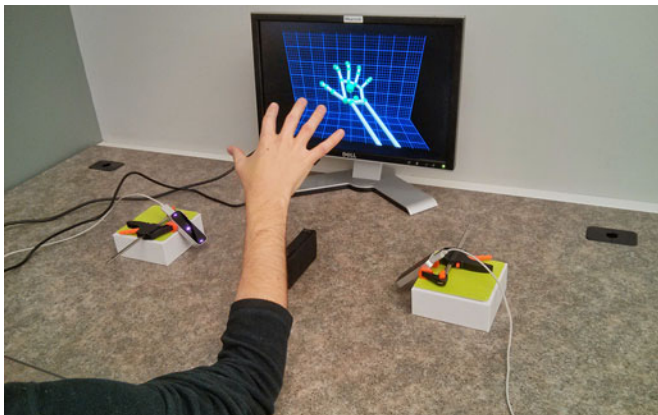
Fig. 1. Example setup used in our lab to capture a single hand pose from two different viewing angles.
