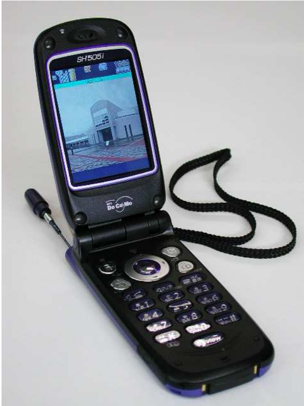
(a) Egocentric Panoramic Browser “ \mu VR 4 U 2 C”: Some mobile phone displays feature autostereoscopic (lenticular) displays. Our dataset and algorithms have been ported to such mobile devices, enabling stereographic viewing of QTVR-like panos and turnos (with quasi-realtime network synchronization). (Developed with Etsuko Nemoto.)
