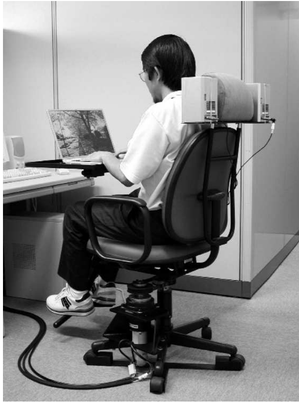
Figure 3. S_{c}h_{a_i}r^e Internet Chair integrated with VR_4U_2C : The swivel chair is a rotary motion platform. The panorama displayed by the laptop computer (with wireless internet connectivity) is proprio-centrally anchored, panning opposite to the chair rotation driven by the servomotor and the soundscape displayed through “nearphones,” loudspeakers straddling the headrest for binaural display without crosstalk. (Developed by the first author and Uresh Duminduwardena with the collaboration of Yamagata University and Mechtec. 55 )
