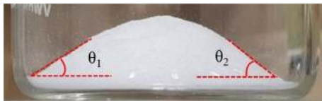
Fig. 5 Experimental AoR of SpheroLac 100
