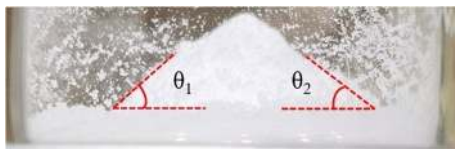
Fig. 6 Experimental AoR of InhaLac 251
