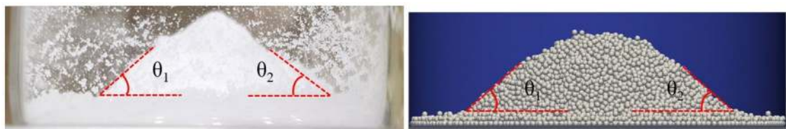
Fig. 28 DEM AoR from the prediction model validated with the experimental AoR of the cohesive powder
