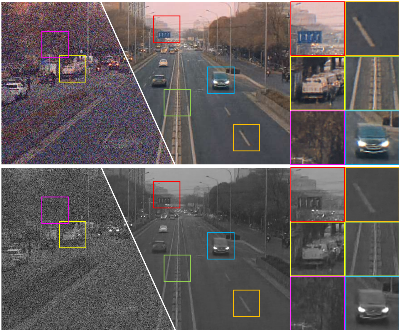
Fig. 11: Our RGB and NIR reconstruction results on a dark video frame captured by our setup at night.
