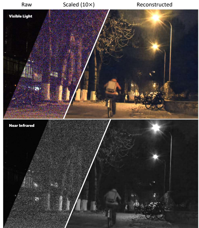
Fig. 1: An example of paired RGB (top) and NIR (bottom) video frame captured computationally by our approach under dark environment. The three segments in each image show the extremely dark raw measurement, linearly scaled version with severe noise and color distortion, and the clean final reconstruction, respectively.
