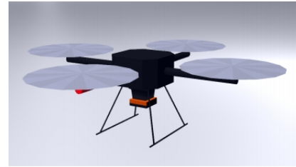
Figure 2. The Hector quadrotor rendered within the Gazebo simulator. Image taken from [12].
